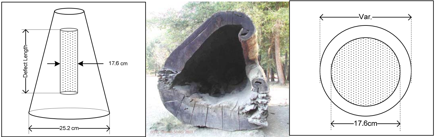
Figure 3.10 - Common type of decay in tree trunk From left to right: Longitudinal sketch of tree defect, Real cross section of decayed trunk, Modeled cross section of decayed trunk
